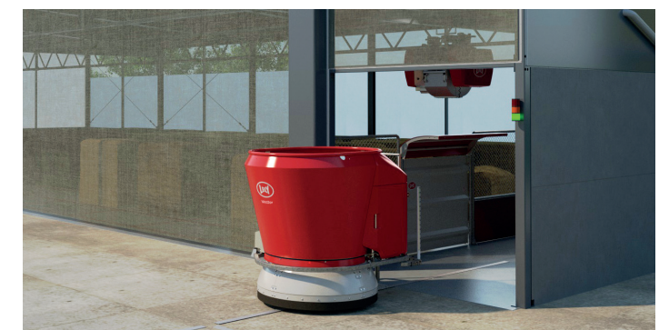
7. Back to the filling & charging station to load a new batch of feed
