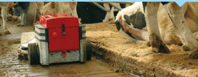
Manure is pushed through the openings of the slatted floors.
